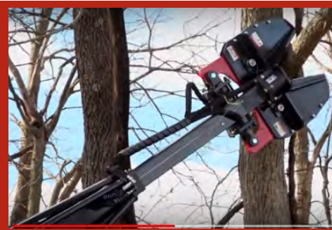
Model TC6451 Telescopic Clipper head with 36" telescope. Ideal for clean-up along ditches and waterways.
