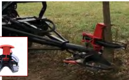
CLAMPER for tree Clipper with Hardened T1 Clamping Blades. Greased Pivot Points. Backstop to prevent tree from falling back Center Load Support on new models. Welded Clamping Cylinder
